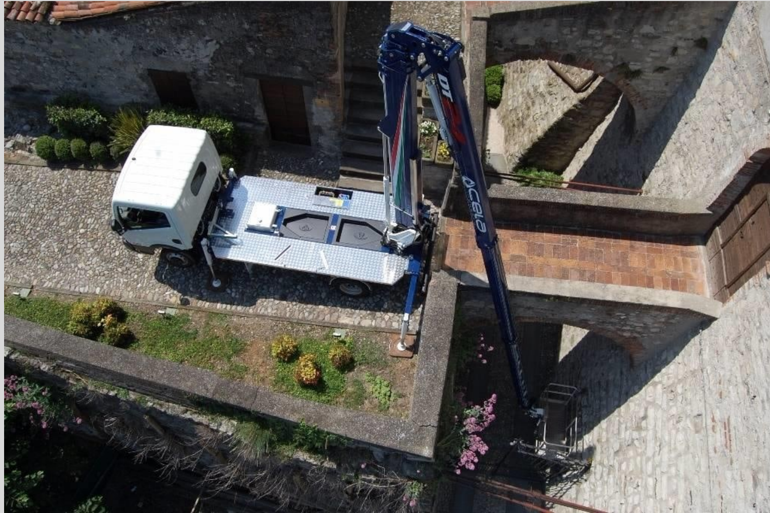
A semicircular working envelope, for outstanding reach below ground level
