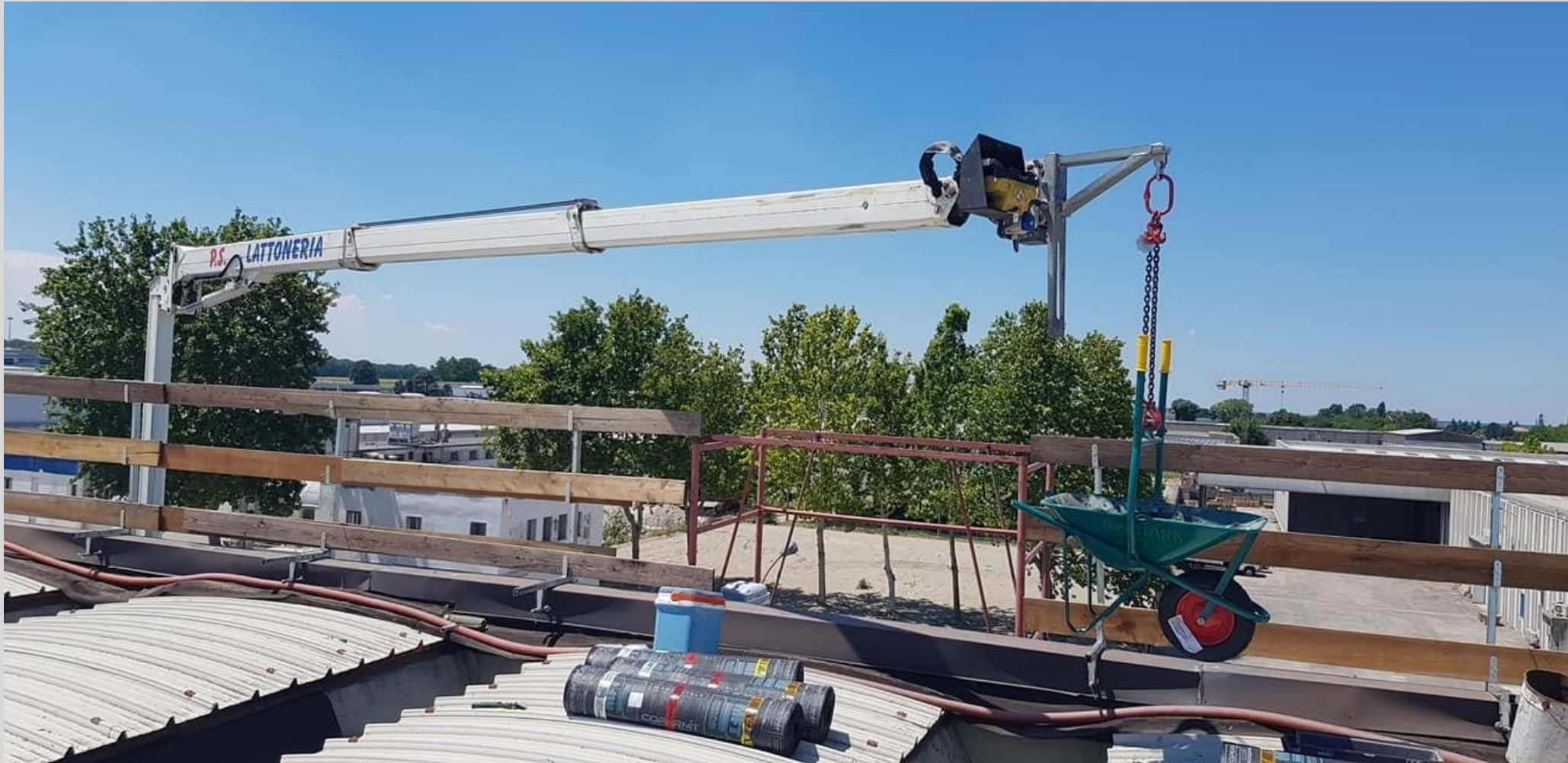
CELA Advanced DT platforms are certified both as aerial platforms and as cranes
