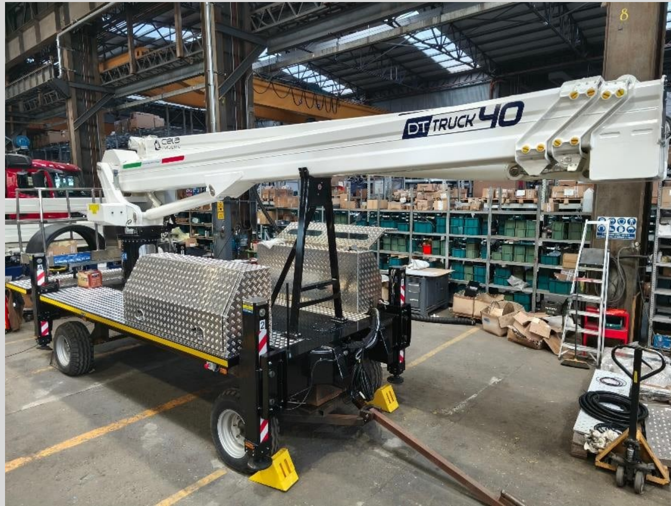
MAD KIT at destination: the CELA upper structure on a locally sourced truck
