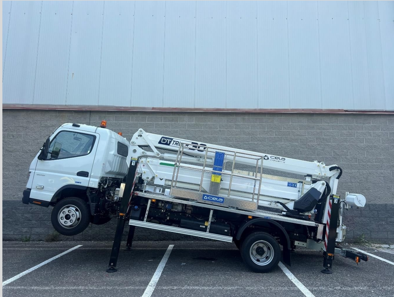
Boxed outriggers let the DT Truck 30 set up on steep slopes
