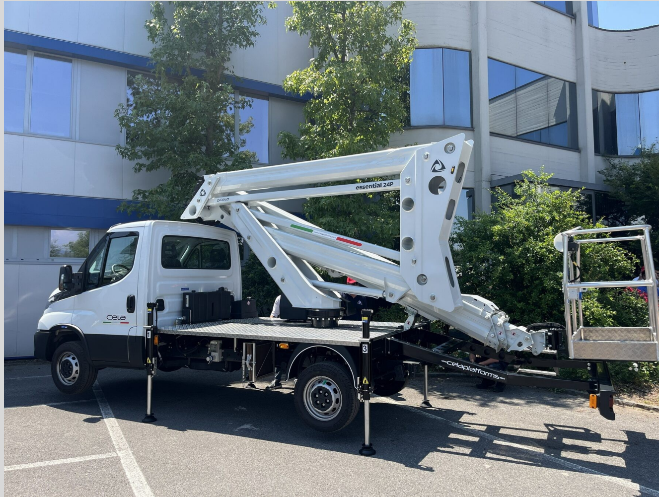
Cela Essential 24P: 78'8" / 24 m of working height from a 3.5 t (7,716 lb) truck, no CDL required
