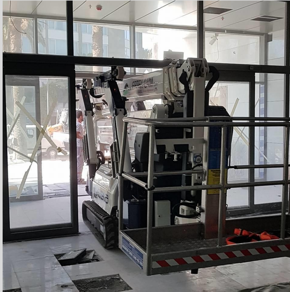
CELA Advanced DT crawlers are narrow enough to drive through a building's door
